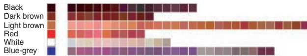
Figure 1. Colour palette employed for colour group attribution. The black colour comprises 15 patches of black hues; dark brown, 10 patches; light brown, 28 patches; red, 9 patches; white, 12 patches; blue-grey, 24 patches. The coloured square at the beginning of the line corresponds to the false colour attributed to the pixels belonging to that colour group.
