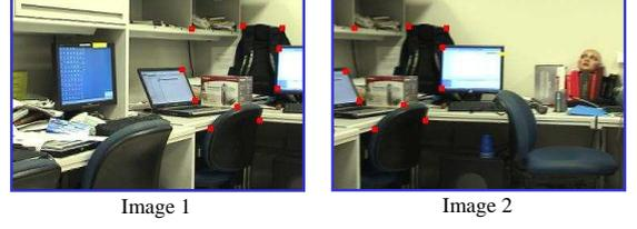
Figure 6: Two images from a pan sequences. The red points represent the correspondences in the images. The rotation axis of this sequence is  $[0.0007, 1.0000, 0.0000]$ , and the magnitude of the rotation angle is  $16.75^\circ$ .
