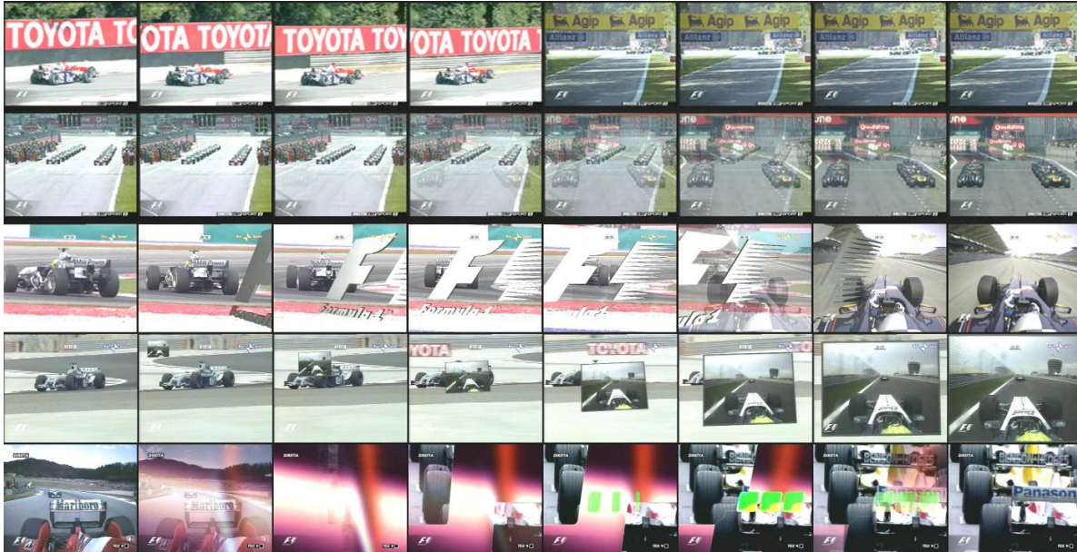
Figure 8. Examples of correctly detected transitions. From top to bottom: cut, dissolve, 3 special edit effects, which are correctly detected because they contain a linear part. For instance, in effect on row 3 there is a dissolve, which is clearly visible at the end. A dissolve is also present at the beginning of effect on the last row. The effect on row 4 shows a linear transform in its last frames.
