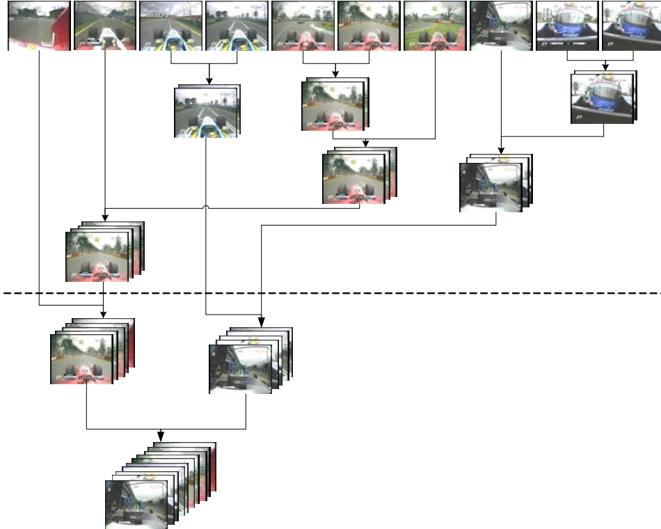
Fig. 1 Example of complete link clustering on 10 sub-shots. The Dunn's Index selected level is shown with a dotted line.
