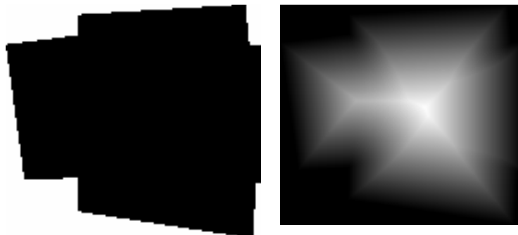
Fig. 4. Example of a mask with its associated distance transform (lighter values mean higher distance from the outside region).
