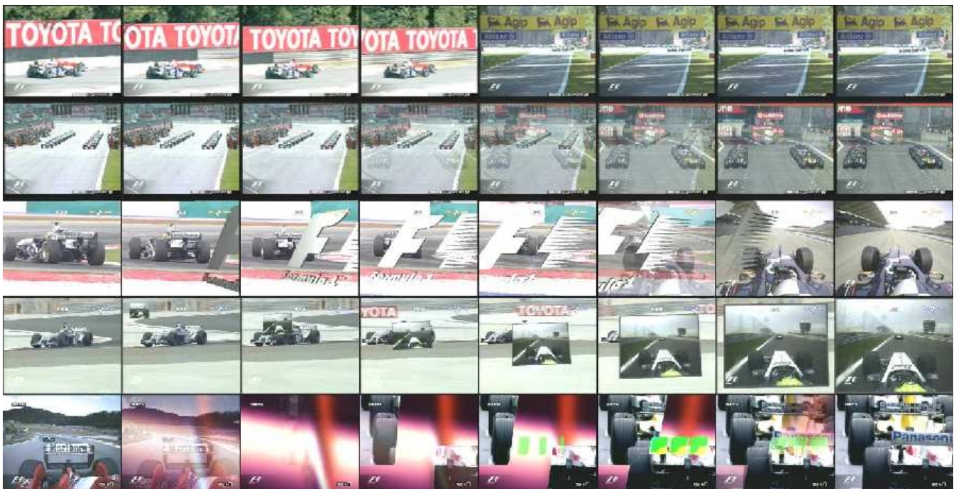
Fig. 4. Examples of correctly detected transitions. From top to bottom: cut, dissolve, 3 special edit effects, which are correctly detected because they contain a linear part. For instance, in effect on row 3 there is a dissolve, which is clearly visible at the end. A dissolve is also present at the beginning of effect on the last row. The effect on row 4 shows a linear transform in its last frames.
