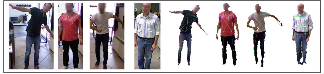
Figure 3: Sample images and corresponding point clouds with the estimated skeletons from the Kinect dataset
