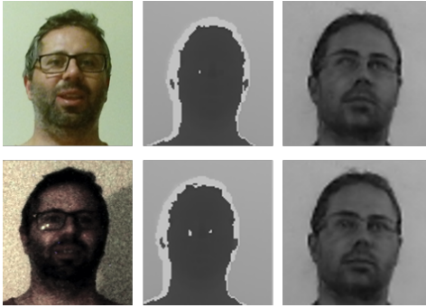
Fig. 2. Example of reliability of the FfD network on depth images. Two consecutive frames have been selected from a sequence with an abrupt illumination change (from light to dark). In the first column the auto equalized RGB, then the corresponding depth maps and finally the FfD reconstruction output.
