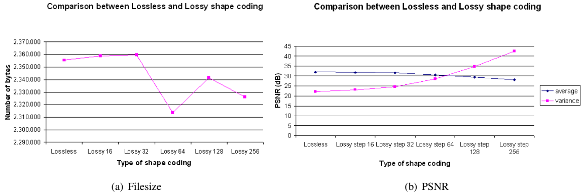
Figure 4. Performance analysis for lossless vs. lossy shape coding.
