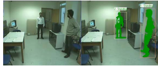
Figure 6. An input frame from a monitored room (left) and the correspondent output of the video surveillance module (right). Blobs, positions, and postures of the people detected are superimposed.
