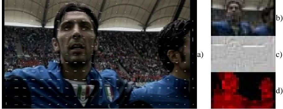
Fig. 1. a) Sample frame with superimposed motion vectors. b) DC Image. c) AC Image. d) Motion Image.
