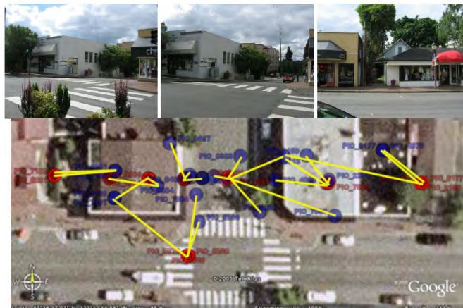
Figure 9.10: Images with unknown GPS location for Final5. Bottom: GPS locations (blue) obtained using our method is compared with ground truth GPS (red). The error in estimates are shown as yellow lines between the ground truth and estimated locations.
