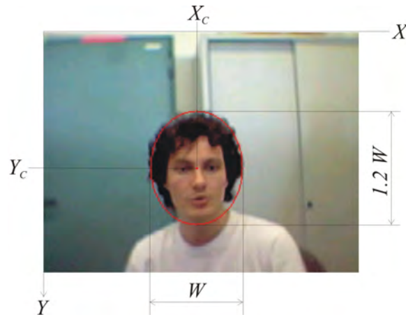
Figure 7.1: The elliptical face model adopted for the head detection. The size ratio and the orientation are fixed.
