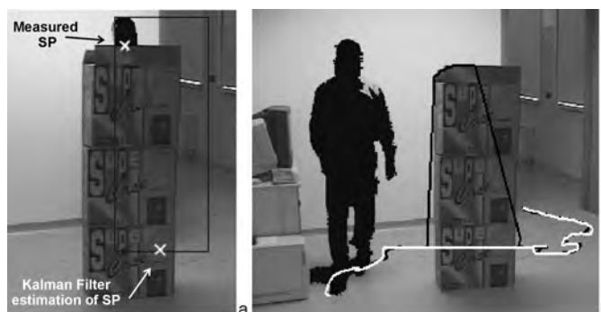
Figure 6.4: SP tracking with Kalman Filters. Trajectories of SP estimated over the blob (black color) and tracked with the Kalman Filter (white color)
