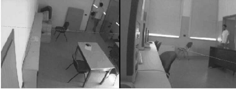
Figure 8.6: The frame extracted from the two cameras during the camera handoff. The lines are the intersections of the floor and the gate plane computed and drawn by the system
