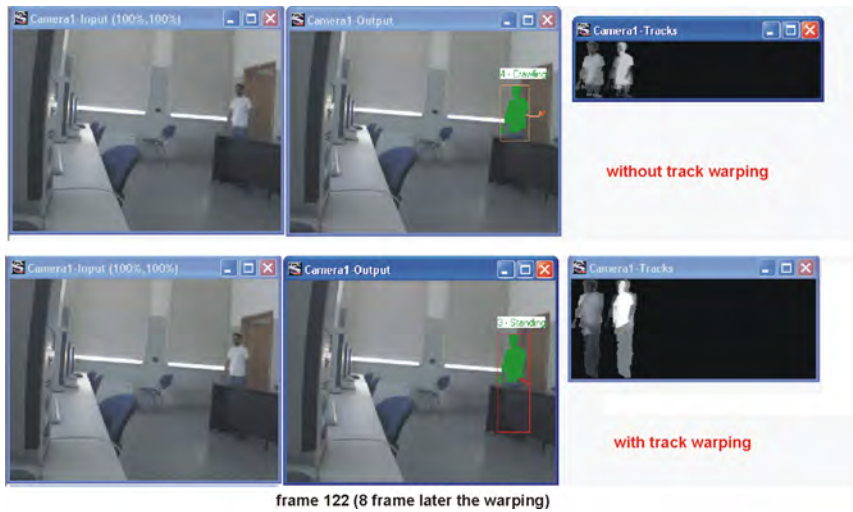
Figure 8.9: Initial occlusion resolved with track warping. a,d: input frames; b,e: output of the posture
