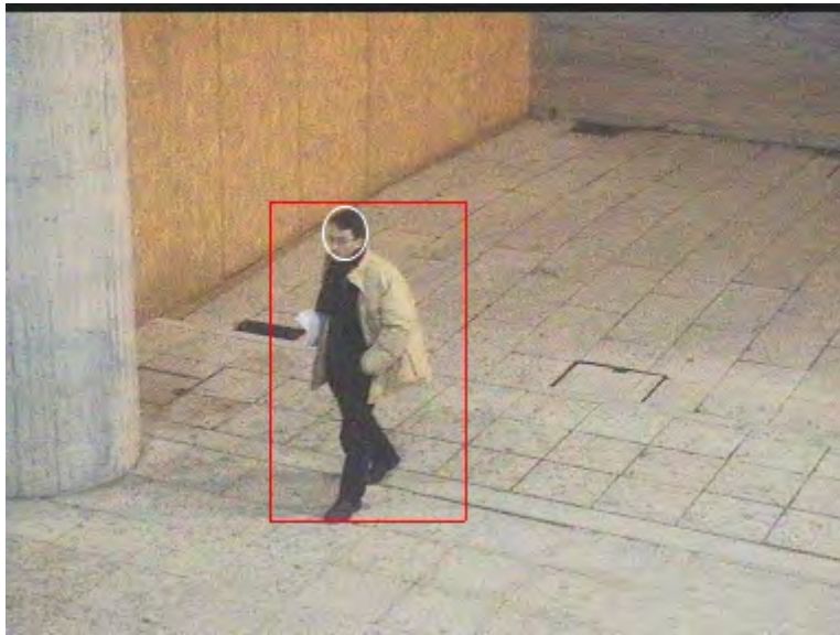
Figure 7.3: Search area obtained with the dynamic mosaicing algorithm and the detected head
