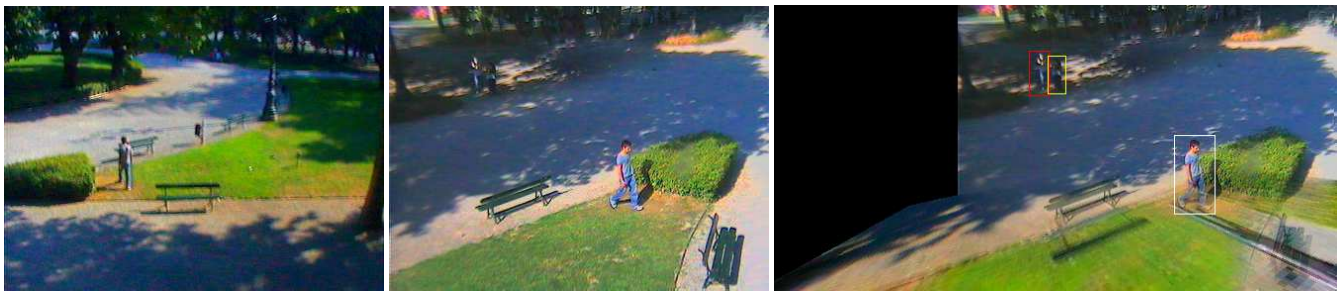
Figure 1: Dynamic mosaic with homography of two partially overlapped cameras. In the homography, note the correspondence between the bench and the person and their distorted shape flattened to the ground plane.
