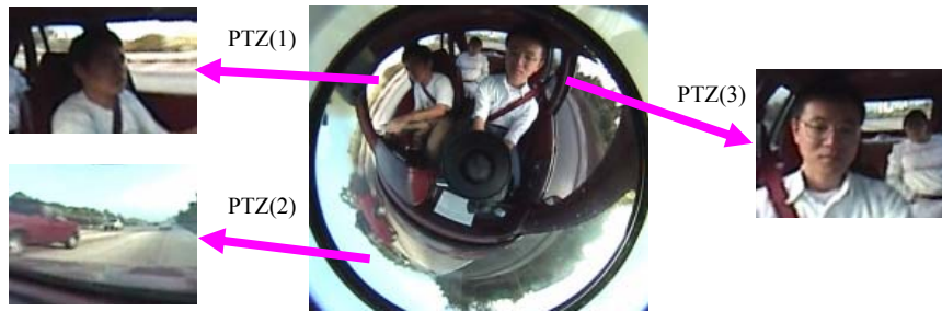
Figure 2. Simultaneous multiple perspective video generation on single omnidirectional video for event analysis. It enables frame-to-frame synchronization by nature.
